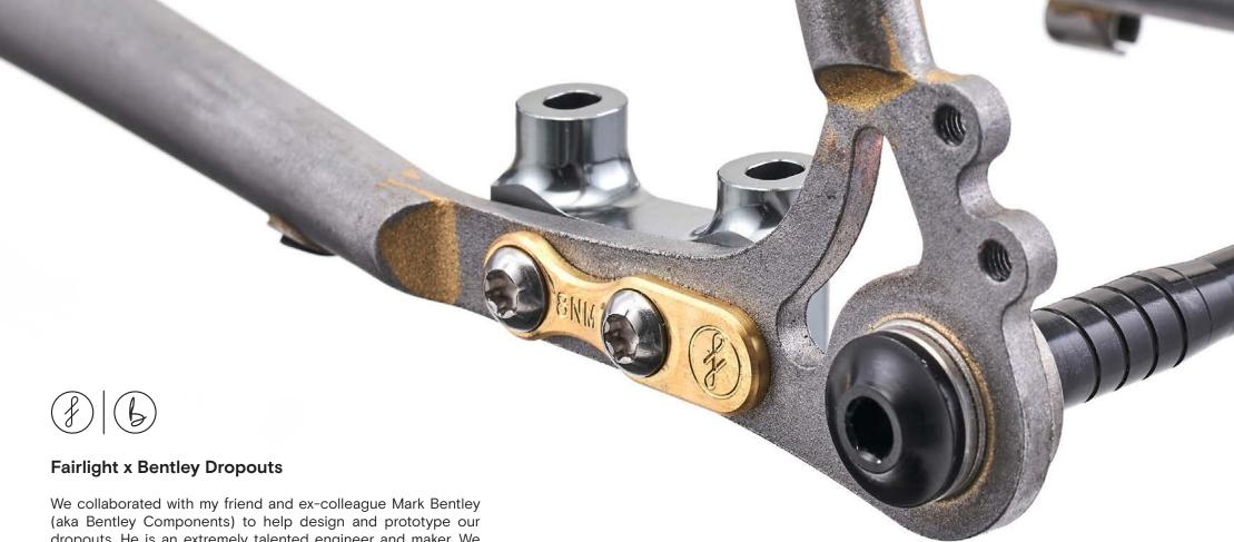
We collaborated with my friend and ex-colleague Mark Bentley (aka Bentley Components) to help design and prototype our dropouts. He is an extremely talented engineer and maker. We use a combination of laser cut steel plate, turned stainless steel inserts and a CNC machined aluminium brake mount to produce a dropout that is light, functional and elegant.
