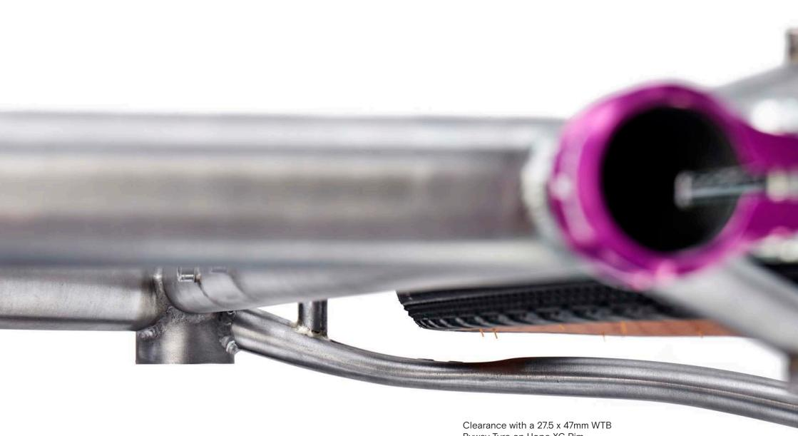
Clearance with a 27.5 x 47mm WTB Byway Tyre on Hope XC Rim
