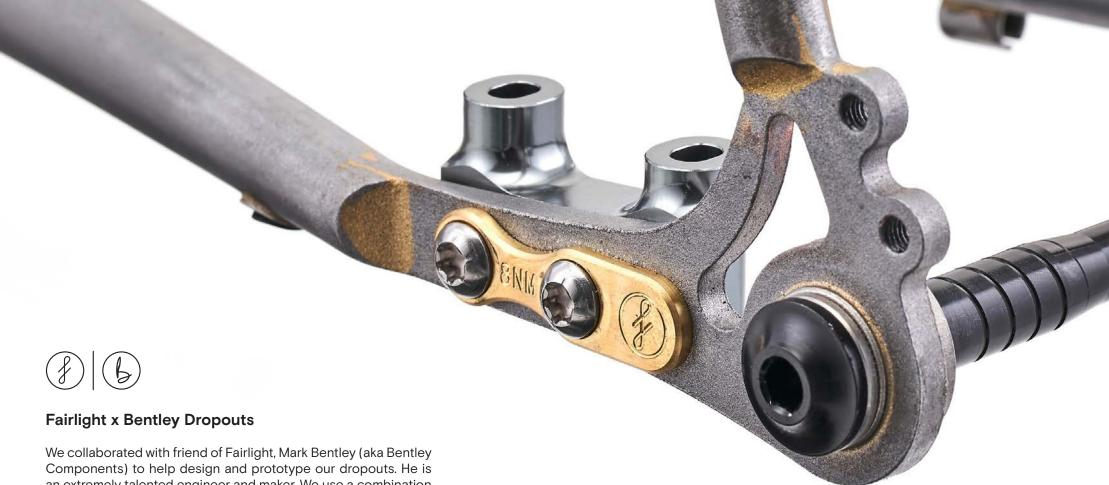
We collaborated with friend of Fairlight, Mark Bentley (aka Bentley Components) to help design and prototype our dropouts. He is an extremely talented engineer and maker. We use a combination of laser cut steel plate, turned stainless steel inserts and a CNC machined aluminium brake mount to produce a dropout that is light, functional and elegant.
