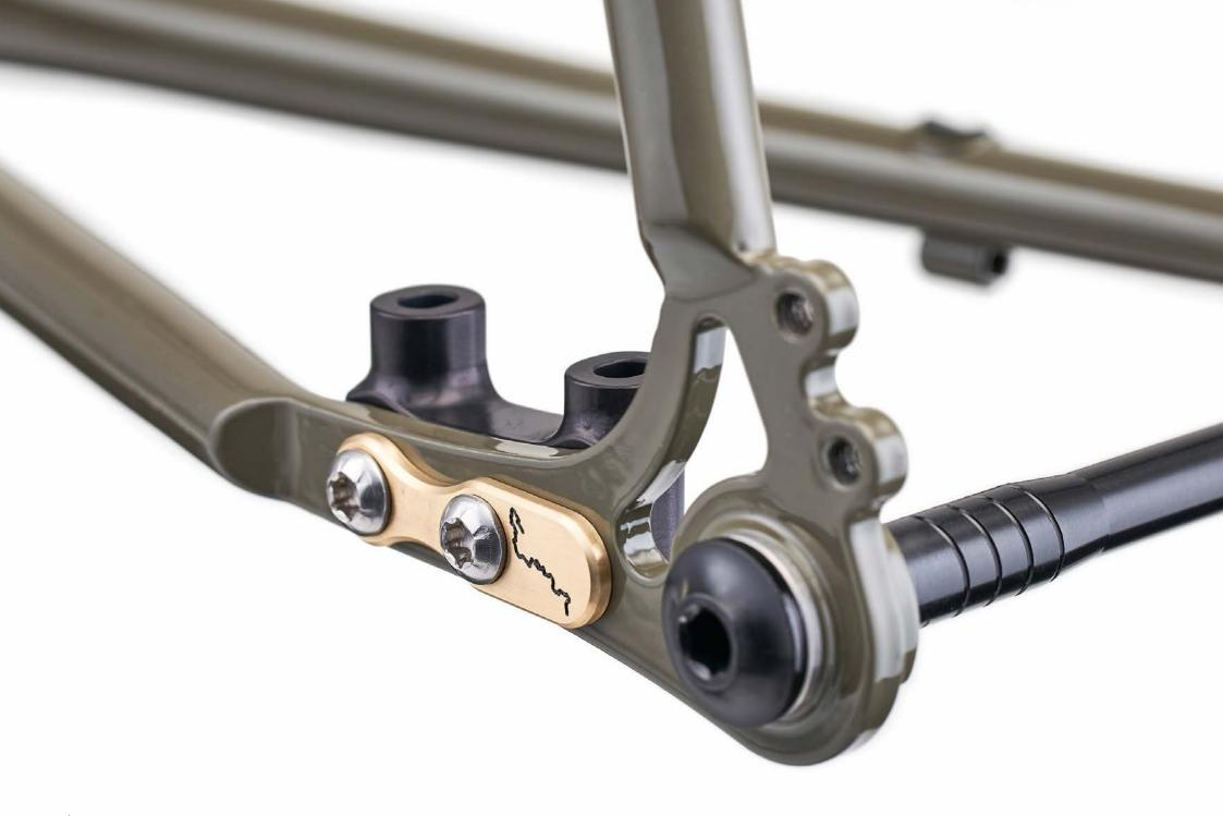
Custom machined parts by Mark at Bentley Components
