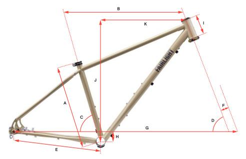
Fork axle to crown measurements are based on: SID SL 100mm with 20% sag = 486mm, SID 110mm with 20% sag = 499mm, SID 120mm with 20% sag = 507mm
